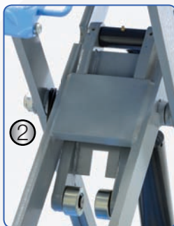
(1) High quality hydraulic cylinder (2) Rocker arm system for powerful lifting (3) Fully loadable, lockable drive-up flaps (4) Extremely flat construction (5) Easy to use control box (6) Teflon sliding blocks (7) Lifting height max. 1 m
