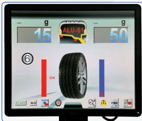
(1) Precise placement of hidden weights using the electronic arm (2) Laser positioning system (3) Quick release nut Ø = 40 mm (4) Electronic measuring arm (5) LED light (6) Large TFT-Colour monitor (7) Quick and easy input by keypad
