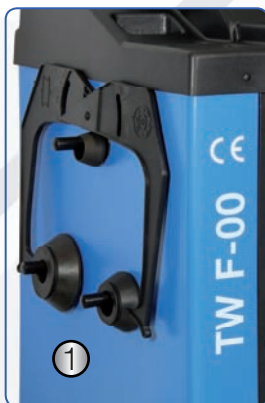
(1) Side holder for centering cones and gauge (2) Integrated distance measurement (3) Quick release nut Ø = 40 mm (4) 15 storage compartments (5) Digital Display (The new, compartment design ensures maximum user comfort and optimal ergonomics)
