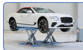
(1) High quality hydraulic cylinder (2) Rocker arm system for powerful lifting (3) Fully loadable, lockable drive-up flaps (4) Extremely flat construction (5) Easy to use control box (6) Teflon sliding blocks (7) Lifting height max. 1 m
