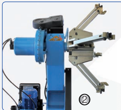
(1) Powerful drive motor with 2,2 kW power (2) Massive and precisely controllable clamping arms with a very large clamping range of up to 42 inches and a maximum wheel diameter of up to 2300 mm (3) Flexible Joystick controller (4) Foot pedals for precise control (5) Flexible bead breaker on mounting arm
