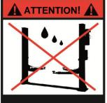
Protect the lift against damp, especially the electrical connections!
