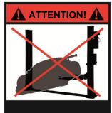
Never try to lift using only one side of the lift!
