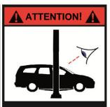
Check vehicle for security shortly after lifting!
