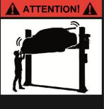
Avoid excessive shaking of the vehicle!
