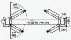
Through experience the required concrete depth (foundation requirement of 200 mm) should be met, this must be checked by the customer. If in exceptional cases the foundation requirement is not met, we offer on page 31 a special solution, which can be used with a concrete
