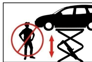
No unauthorized persons under the lift when in use
