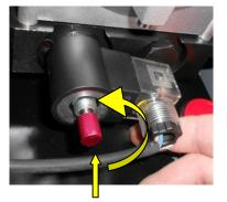
When opened the platforms will drop to the next safety catch, then close the valve and shortly open the two ball valves to release the pressure. These steps must be repeated to achieve the perfect level.
