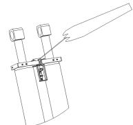
4. Screw loose the core of solenoid unloading valve fixed on the hydraulic block.
