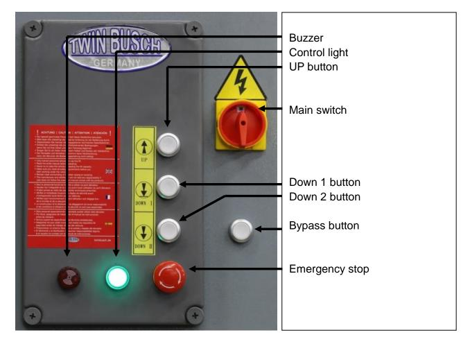
After switching on the main power a green light should be seen to show that the unit has power.
