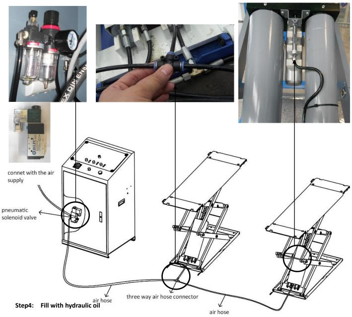
Fill the oil tank with 15 liters of hydraulic oil. Level can be checked using the dip stick attached to the lid
