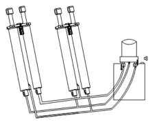
2. Connect the optional hand pump to hydraulic block at the point where the removable plug used to be fitted.
