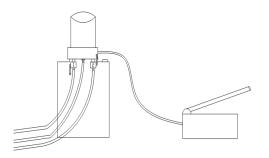
3. Press the handle of the optional hand pump to raise the platform to have the safety teeth unlocked. Then, pull up the safety teeth with steel rope to release the safety lock.
