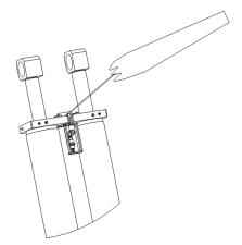
2. Screw loose the core of the solenoid unloading valve fixed on the hydraulic block.
