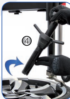
(1) Help-arm for professional use (2) Mounting head (3) Comfortable and clear tire inflator (4) Self centering wheel mounting system (5) Wheel lifter
