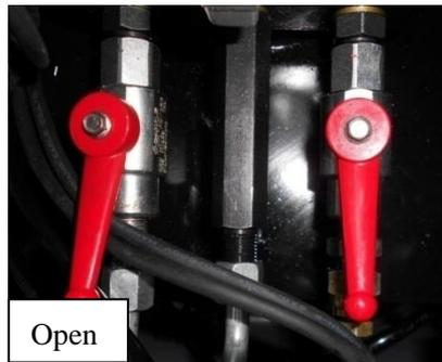
8. As soon as the platforms have roughly the same level, raise about 20 cm and open the manual release button. This must be pressed in and turned left to open.
